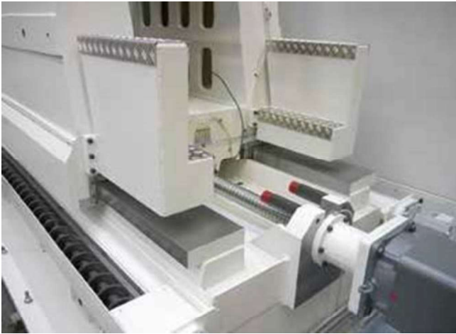
2 Z-axis and stands of a flat-guided machining centre. The extremely powerful dimensioning of the components is aimed at eliminating vibrations across the entire system (© Burkhardt+Weber)
