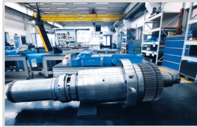
DEFECTIVE MAIN SPINDLE BEFORE DIAGNOSIS.
