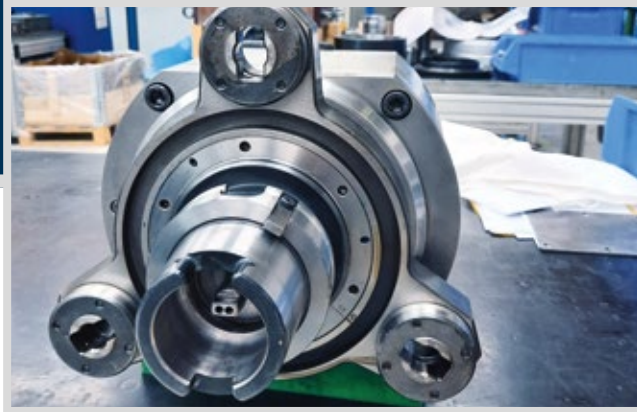
FACING HEAD BEFORE REPAIR.
