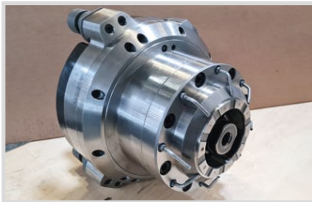
REPAIRED TURNING TOOL ADAPTER.
