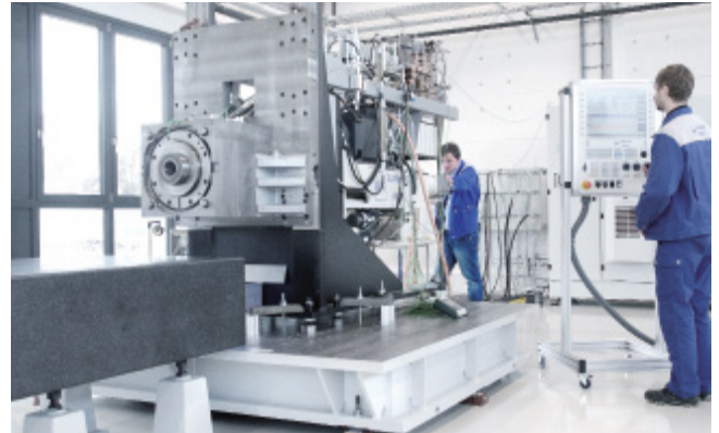
D160 quill unit on test bench.
