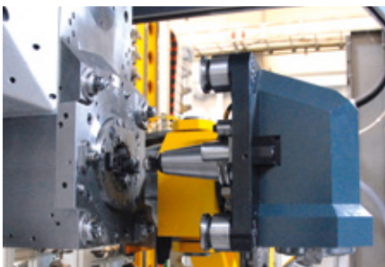
The tool changer transfers the tools (max. 75 kg) to the main spindle. The turning tool holder is also loaded from the magazine to the hydraulic clamping.
