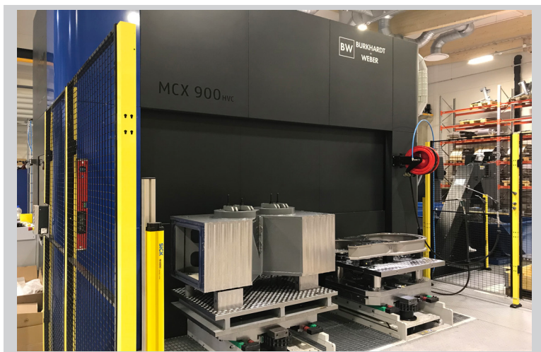
Machining of general frame parts & driving components on a MCX 900HVC
