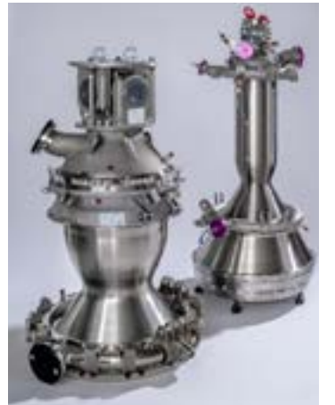
ArianeGroup produces the thrust chamber for the engines of the Ariane rocket carrier in Ottobrunn.
