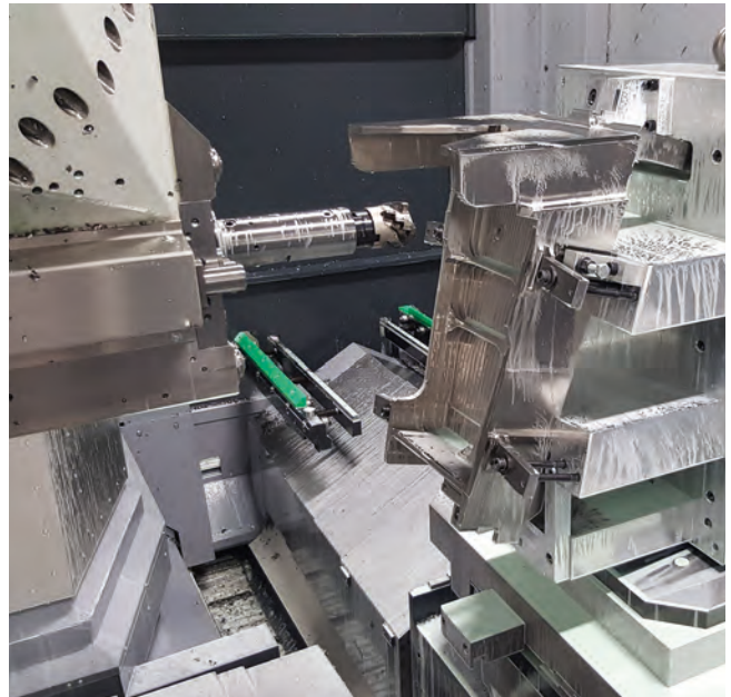
Structural wing part for a business jet from a titanium forging from voestalpine BÖHLER Aerospace GmbH & Co KG.
