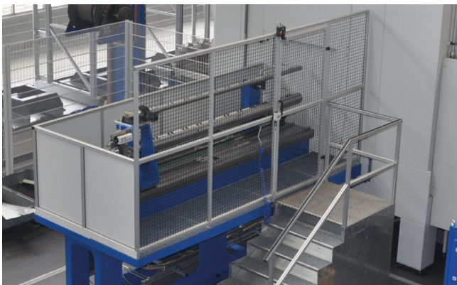
Automatischer Bohrstangeneinschub. – Made by BW.
