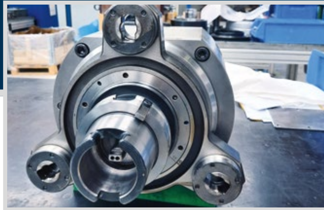
FACING HEAD BEFORE REPAIR.
