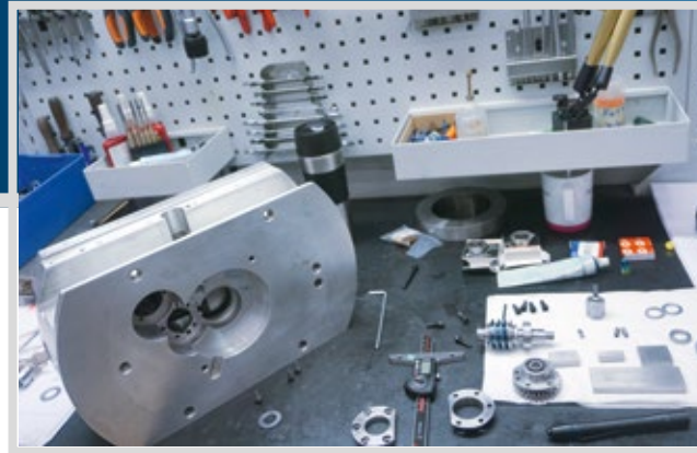
REPAIR WORKS ON A FACING HEAD.
