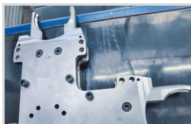
TOOL DOUBLE GRIPPER COMPLETELY ASSEMBLED.
