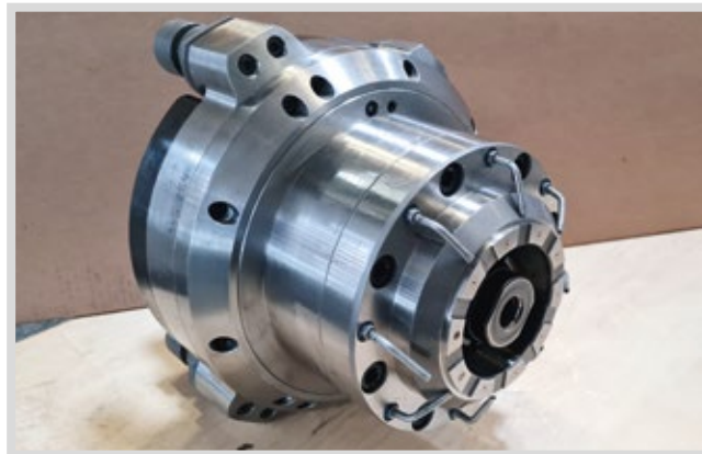
REPAIRED TURNING TOOL ADAPTER.
