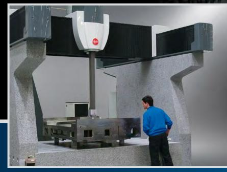
Ideal conditions: High-precision machining at BW at our air-conditioned manufacturing facilities; temperature controlled within  $\pm$  1°C. This complements the thermo-symmetrical structure of our coordinate measuring machine (CMM), also located within the identical temperature conditions.
