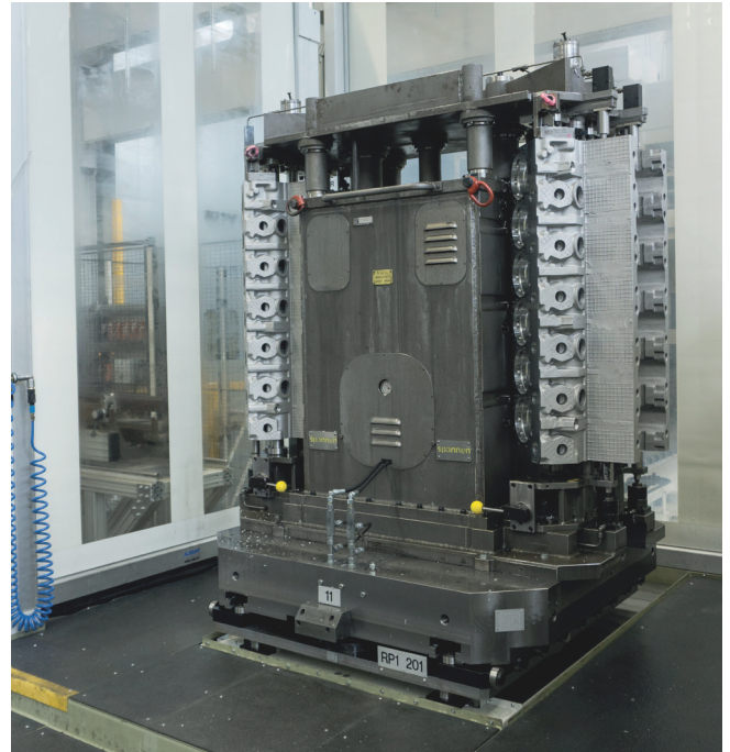
Tooling stations with fixtures and workpieces; boring bars can also be inserted.
