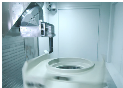
For the „MACHINE CHECK“, turning and milling operations were performed on a cast-iron table housing. The rigid turning tool holder ensures a very stable cut. (cutting parameters for turning: v_1 = 0,6 mm/revolution; v_2 = 200 m/min; a_p = 6 mm).
