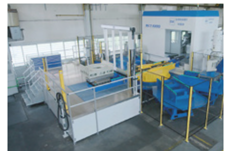
All pallets are manufactured at BW. A double pallet changer comes standard. An expanded version that handles up to six pallets is available.
