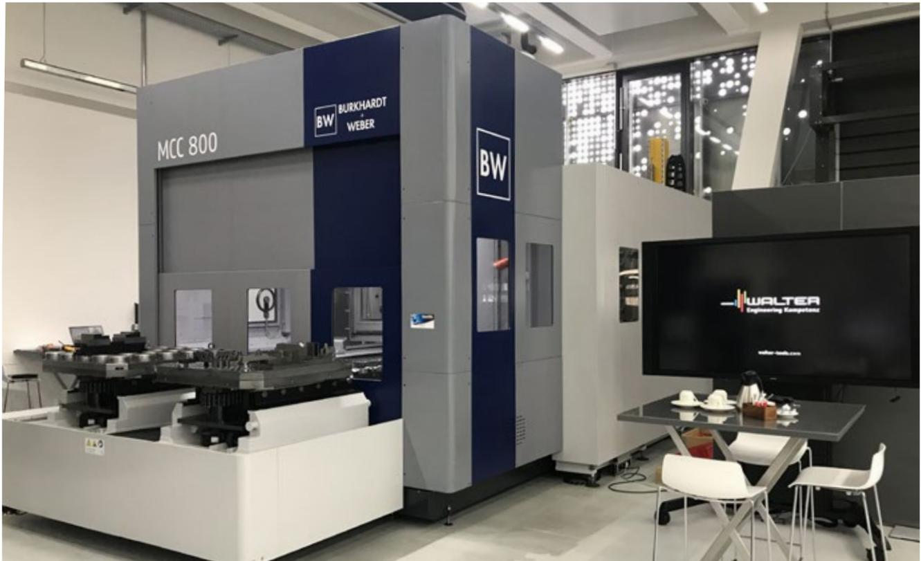
A special centerpiece of the MCC 800 HVC at BURKHARDT+WEBER is the new generation of the tilting head. The existing HVC unit had to be adapted to the new space requirements of the MCC machine.
