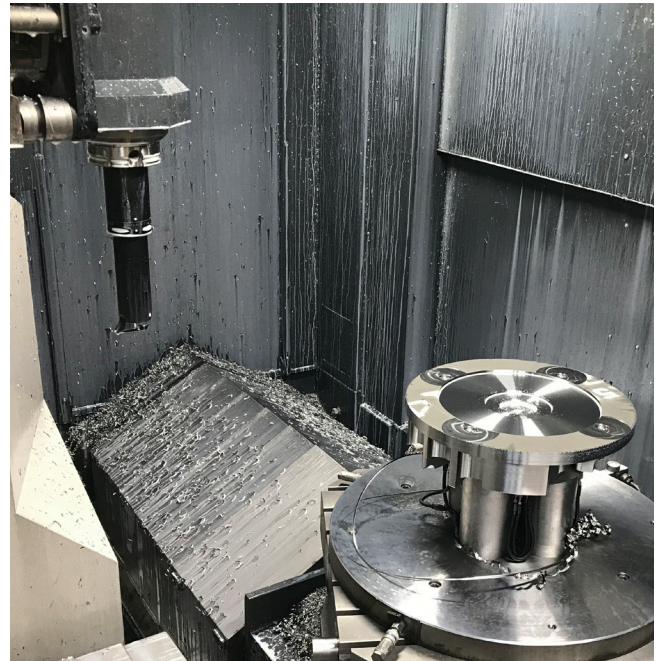
Multitasking machining of characteristic milling heads on a MCT 800
