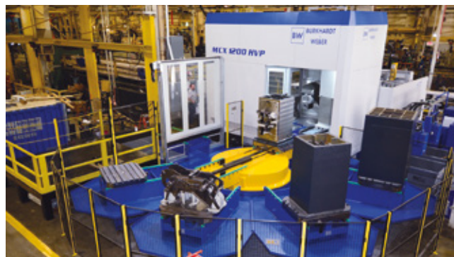
A six-pallet station for automated loading/unloading of parts enables lights-out machining. This configuration can carry 30 parts: five on each tombstone, using the four sides and the top for the fifth workpiece.
