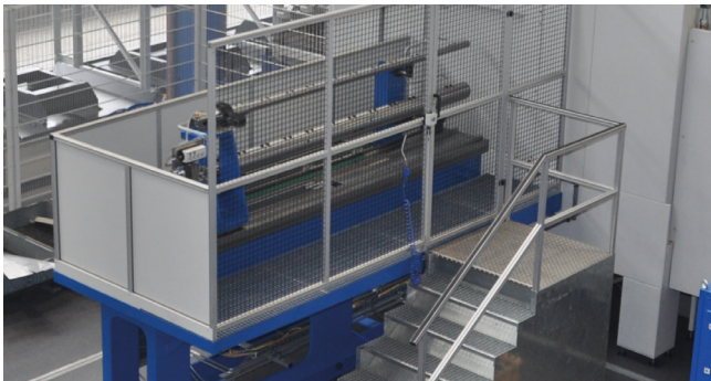
Automatic Line-boring Bar Feed Station – Made by BW.
