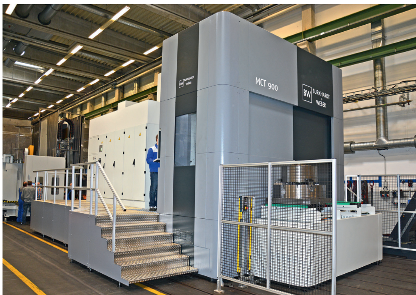
1 Technology integration of milling, drilling, and turning in a single high-performance 5-axis gearbox centre: the new MCT 900 milling-turning centre of Burkhardt + Weber
