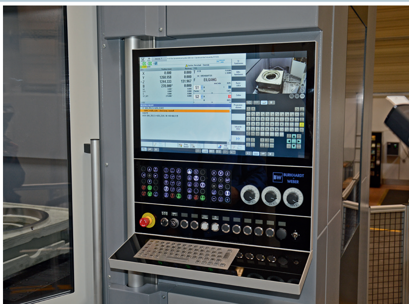
3 Poised to set a new standard for ease of operation: the new 24" smart panel for intuitive machine operation (image: Hanser)
